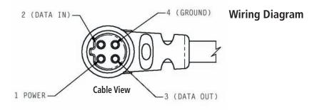
Interface formats are selected from the Setup 'Interface Page' on page 55 of this manual. See also page 68 for using the Rino with MapSource. The input/output lines on your Rino unit are RS-232 compatible, allowing easy interface to a wide range of external devices, including PC's, differential beacon receivers, marine autopilots and /or a second GPS receiver.
